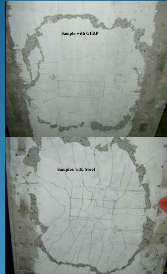
Use of FRP as reinforcement bar in concrete sheet samples (from http://www.bpcomposites.com )
