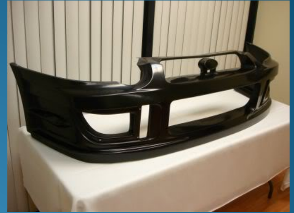
FRP as bumper illustrating material deformability (From http://www.aliexpress.com )
