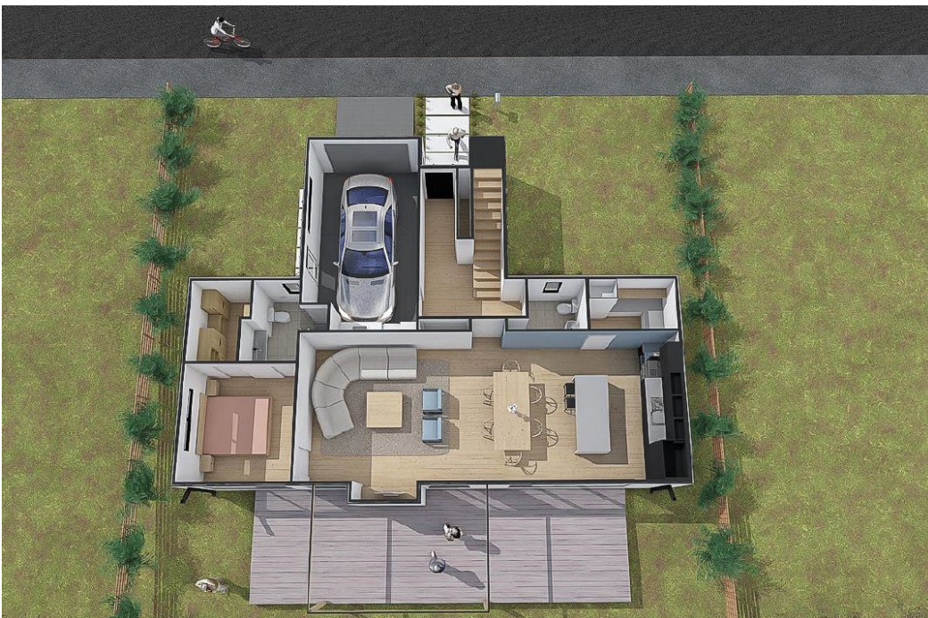
Figure 2. Typical cut-away plan view showing house ground floor and various 3D objects to be photo rendered. Image: A. Jensen.
