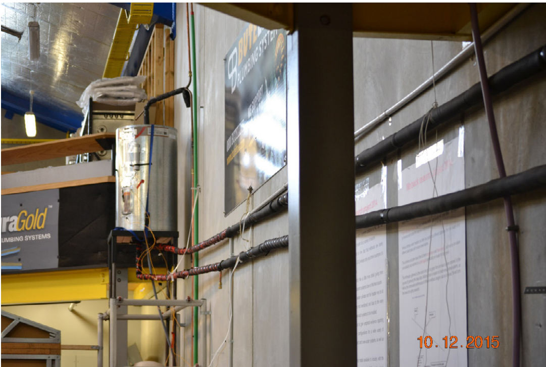
Wetback pipes at 10 m distance, conventional connections.
