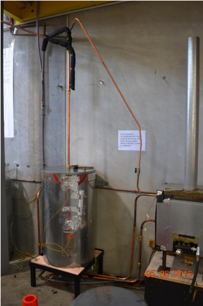
Figure 18. Cylinder below heater level. This test used a vent from the high point of the flow pipe connected to the cylinder vent, which allowed some circulation.
