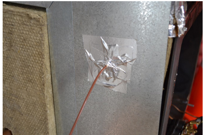
Other thermocouples attached to pipework. Thermocouple in heater to check temperature inside heater was constant.
