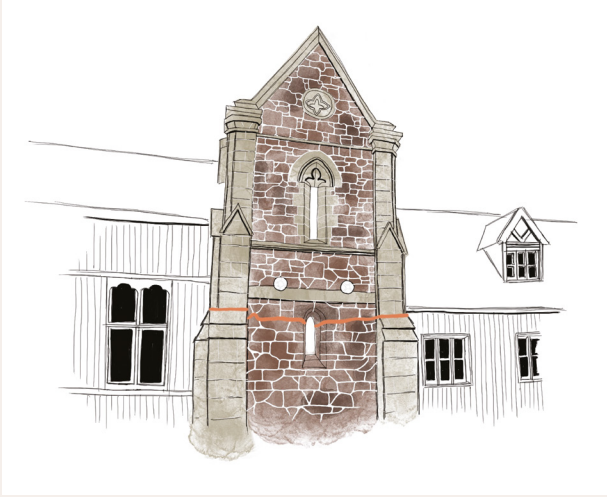
Figure 11. The substantially reinstated Durham Street Tower (above the line indicated). Drawing: Tanya Bezuidenhout
