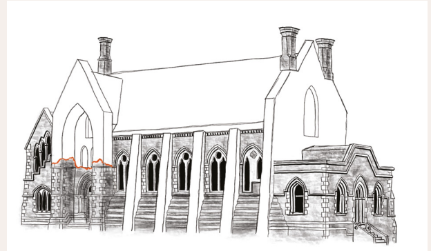
Figure 14. The reinstatement of material between the buttresses 'weaves' new and old elements together, respecting the overall history of the Stone Chamber. Drawing: Tanya Bezuidenhout
