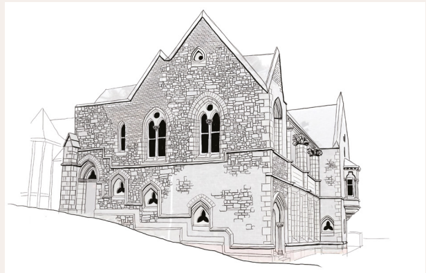
Figure 10. Perspective of Bellamy's illustrating selective reconstruction with new masonry. Drawing: Tanya Bezuidenhout
