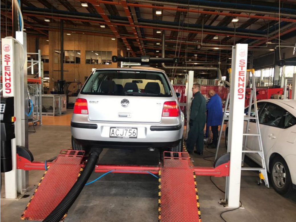
Figure 2. Emissions test setup for Volkswagen Golf 2001.
