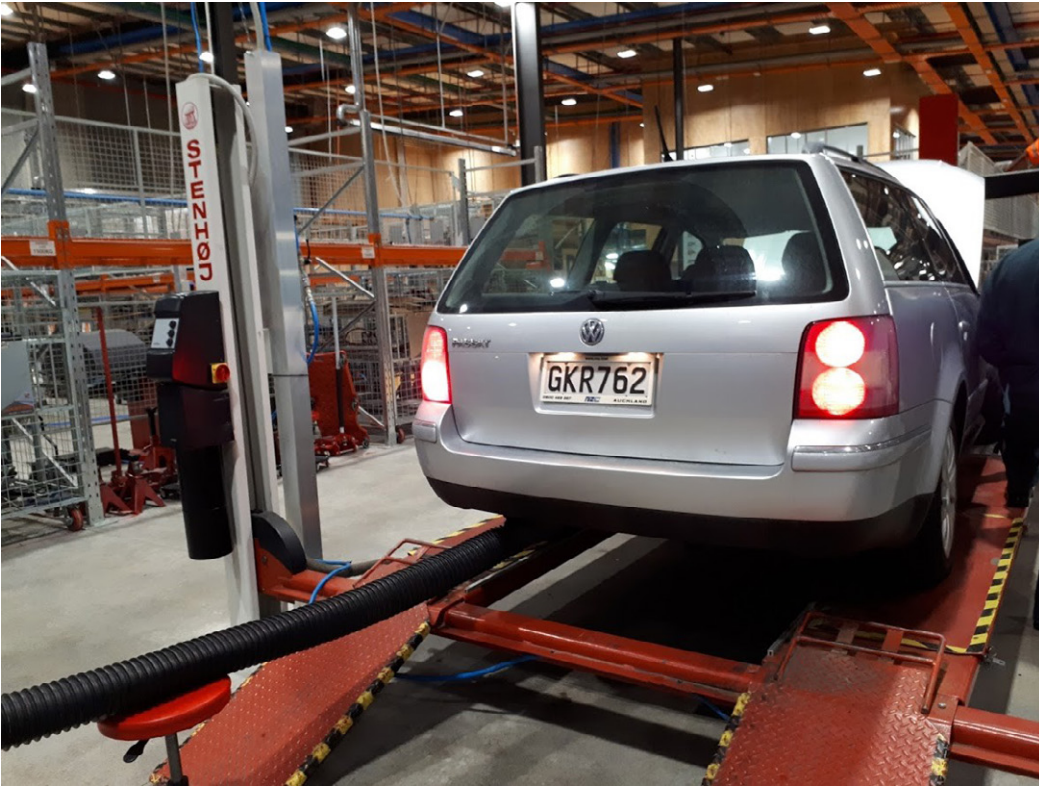
Figure 5. Emissions test setup for Volkswagen Passat 2006.
