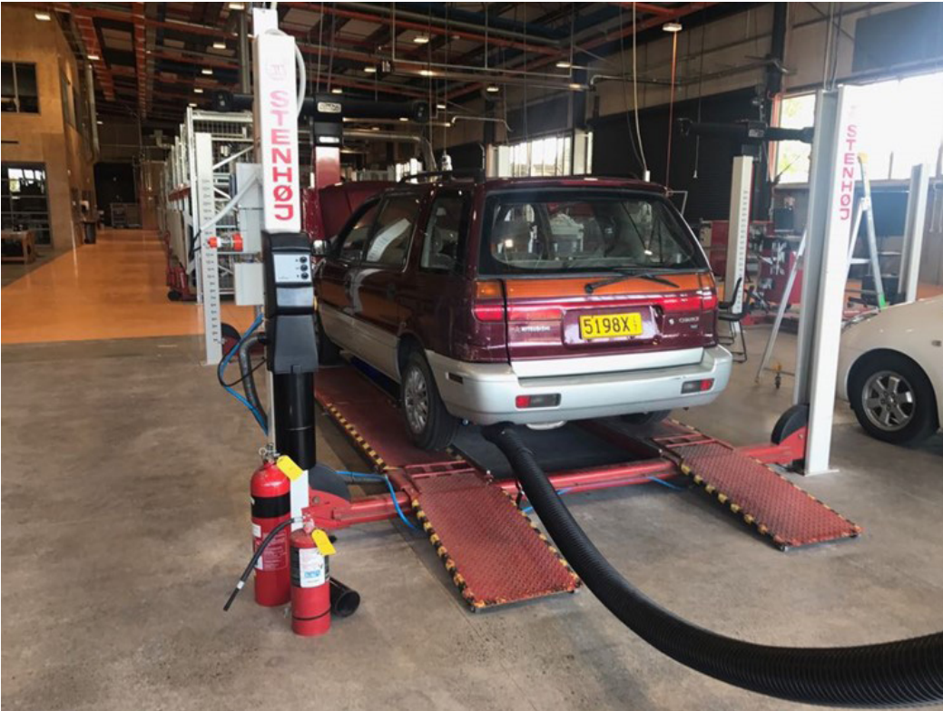
Figure 3. Emissions test setup for Mitsubishi Chariot 1994.
