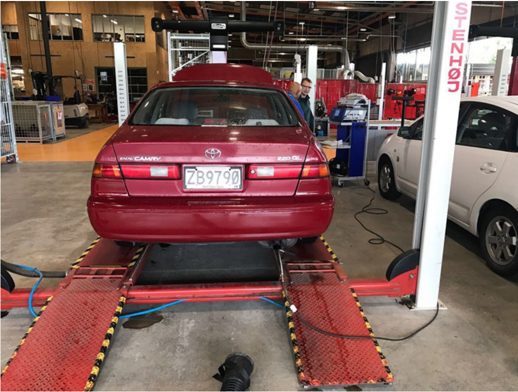
Figure 1. Emissions test setup for Toyota Camry 2000.
