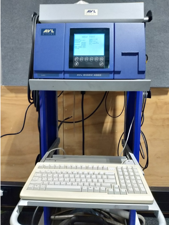
Figure 6. Emissions test setup – the AVL 4000 tester.
