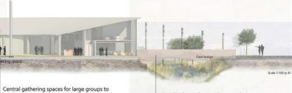
gather on top of a compacted base that provides effective drainage run off to the inlets/
