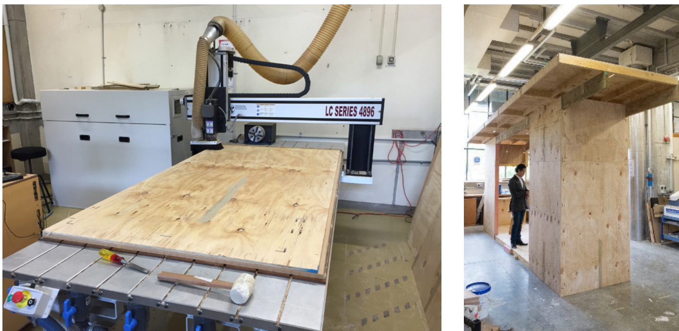
Figure 5. Left: Flat-pack components being fabricated at University of Auckland on a CNC router. Right: The EDFAB 2.0 wall-to-ceiling prototype at the University of Auckland, November 11, 2015.
