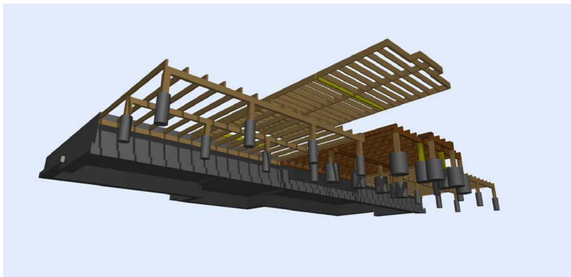
Figure 11. BIM model of dwelling highlighting the elements required in a timber sub floor in their context. (Source: Richard Kelly, Unitec, 2013)
